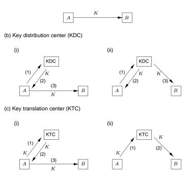
Figure 13.1: Simple key distribution models (symmetric-key).
